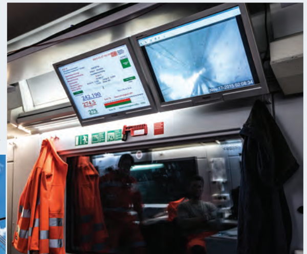
High speed trials in the Gotthard Base Tunnel were conducted during November and December 2015 using the ICE-S test train on hire from Deutsche Bahn. This set a new Swiss record when it 274.5 km/h at 02.15 on November 17 2015 (right).
