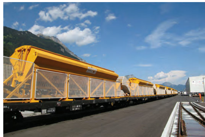
The concrete train spends two shifts in the tunnel. During the third shift it returns to the base at Erstfeld for a thorough clean before reloading. Facilities at Erstfeld include the cleaning and loading plant (left). About four or five days of material will be stocked on site to keep the train replenished.
