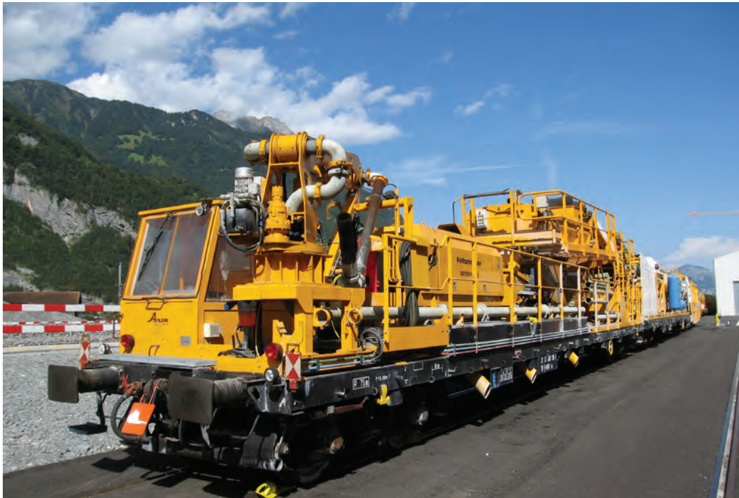
Leading the 500 m long concrete train is the pump wagon, followed by 'Helvetia', the machine at the heart of the concrete train that mixes the materials for the track slab laid in the tunnel.
