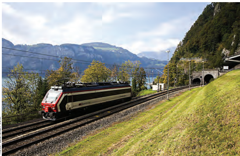
All trains operating over the Gotthard line must now be equipped for ETCS Level 2, including SBB's Roger 1000 infrastructure monitoring vehicle.
