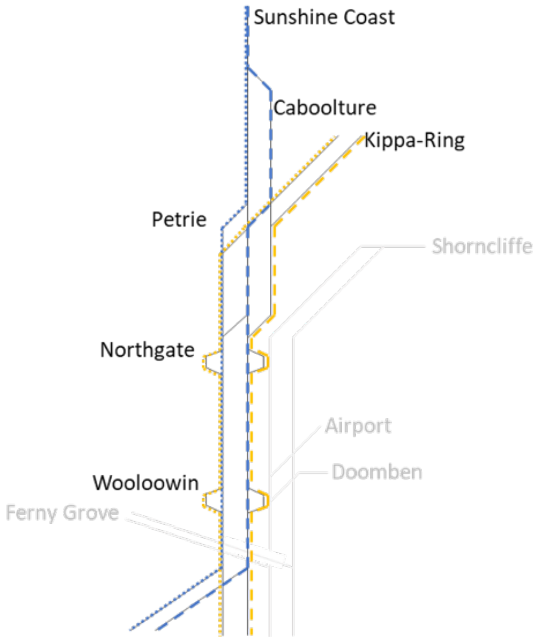
Figure 9: AM peak flows with the Northgate and Woolloowin configuration. Up to 15tph from each of the Sunshine Coast and Kippa-Ring lines can be operated on the single track by running express, and then splitting through the Mains and Subs. The lower contra-peak service level can fit on one track between Northgate and Petrie. NB: the arrangement at Petrie is not shown accurately here, as the junction allows conflict-free movements.
