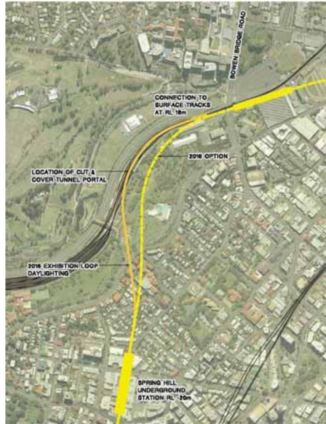
Figure 5-5: Possible alignment for exhibition loop daylighting
